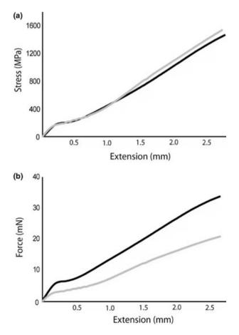
**Fig. 3:** Tensile tests for single exemplar fibers from spiders fed flies (gray line) and crickets (black line). (a) Stress-extension characteristics are nearly identical for major ampullate silk from the two treatment groups. (b) However, the larger diameter of silk spun by spiders in the cricket treatment results in their fibers breaking at approx. 65% greater force than fibers spun by spiders in the fly treatment
